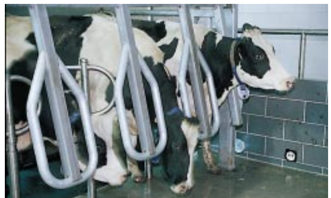
The open bottom neck rail design promotes free cow flow allowing a cow to enter the stalls naturally with her head down. This reduces load time and increases throughput.
