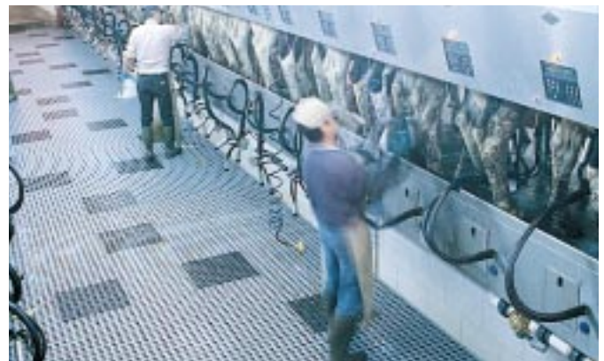
The powered index system uses gentle pressure to automatically position cows correctly for more efficient milking.
